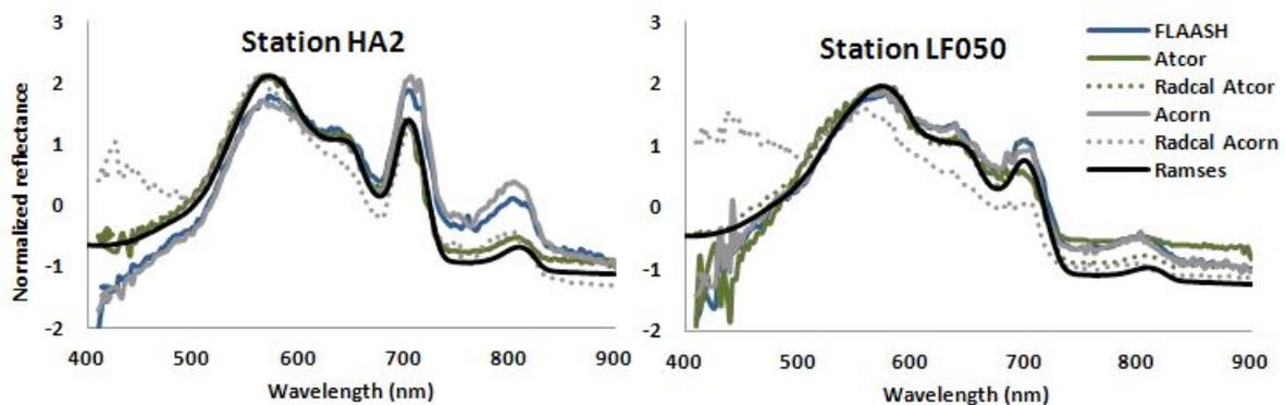
Figure 4. Direct comparison between the atmospherically corrected normalized reflectance spectra and ground reflectance spectra obtained using Ramses field spectrometer in two field stations in the Haapsalu Bay.
