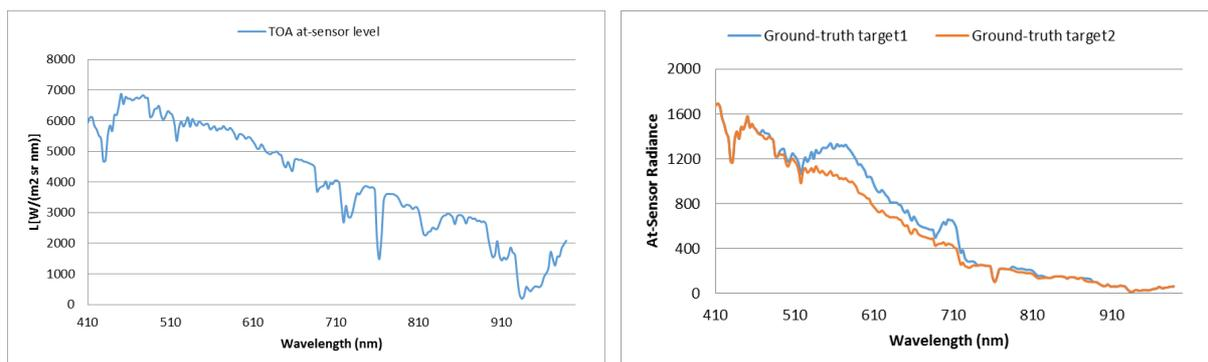
Figure 1. MODO modelling results. First image shows the top-of-atmosphere radiance without introduced ground through spectra. Second image shows the MODO modelled at-sensor radiance spectra for two different field stations.
