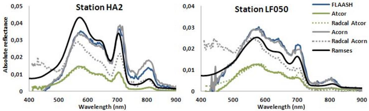
Figure 3. Direct comparison between the atmospherically corrected absolute reflectance spectra and ground reflectance spectra obtained using Ramses field spectrometer in two field stations in the Haapsalu Bay.
